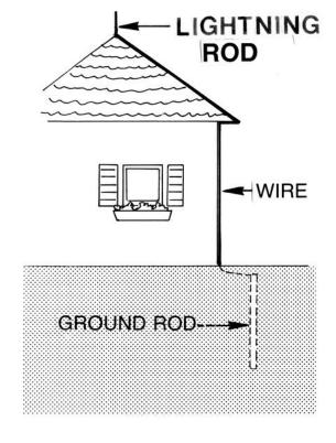
Ben hoped lightning would hit the rod instead of the house. The electricity would travel down the wire to the ground.
